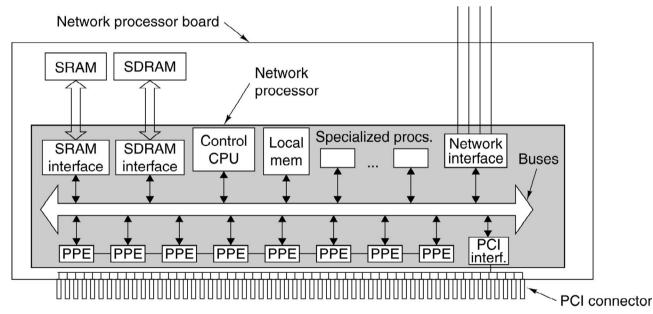
Note the multiple PPE (Packet Processing Engines). Each is a specialized core with a dedicated task; the set forms a packet processing pipeline.
