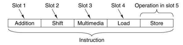
The TMS3260 implementation runs at 250 MHz. Since it can issue five operations per clock cycle, it has an effective maximum rating of 1250 MIPS.
