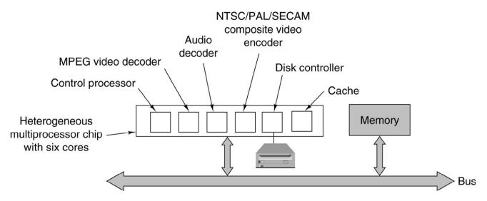
This design uses multiple cores on a single large chip. A **core** is a large circuit, such as a CPU, I/O controller, or cache, that can be placed on a chip in a modular way. Some modern processors are **dual–core** in that they have two cores, each being a full CPU.
