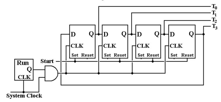
When the run flip-flop is set, the clock pulses get through to the state register and cause it to count.
