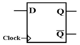
The characteristic table for the D flip-flop is so simple that it is expressed better as the equation Q(t + 1) = D. Here is the table.
