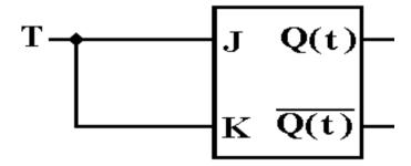
As an SR flip-flop. Just never use J=1 and K=1 as simultaneous inputs.
