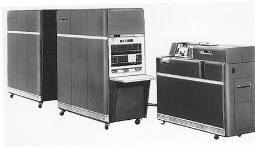
Figure: The IBM 650 – Power Supply, Main Unit, and Read-Punch Unit Source: Columbia University [R41]
