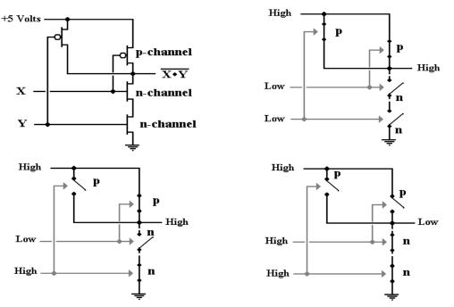
Note that the output is low (logic 0) only when both of the inputs are high. If one or more of the inputs is low (logic 0), then one or more of the NMOS transistors (labeled "n-channel") will be non-conductive, acting as an open switch, and the output is high (logic 1).
