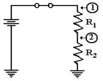
In general,  $E_2 = (E \bullet R_2) / (R_1 + R_2)$ , the value being somewhere between the full voltage and ground voltage, defined to be zero.
