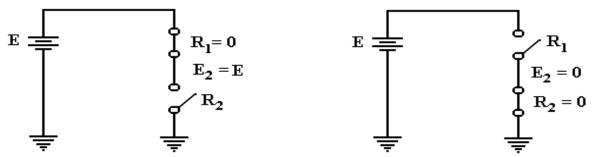
When the top switch is closed ( $R_1 = 0$ ) and the bottom switch is open ( $R_2 \neq 0$ ), the voltage  $E_2$  is the full voltage. When the top is open and the bottom closed,  $E_2 = 0$ .
