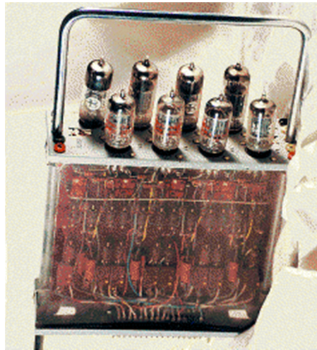
Single Digit from a Burroughs 205 Accumulator, circa 1954.
