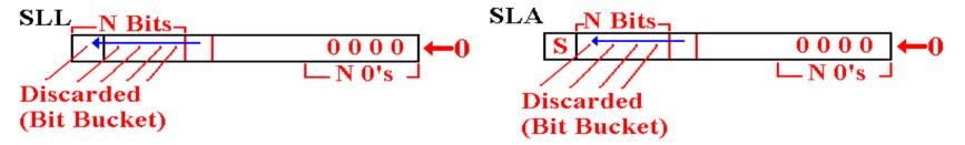
For an N-bit logical left shift, bits 0 through (N - 1) are shifted out of the register and discarded. Bits 31 through (32 - N) are filled with 0.
