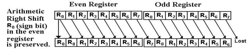
If the above example were a logical double right shift, a 0 would have been inserted into the leftmost bit of the even register.
