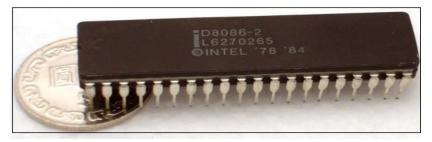
The complexity of the IA-32 series processors grew as the series evolved, and the number of pin-outs required grew with it. By the time of the Intel 80486, a DIP arrangement was
