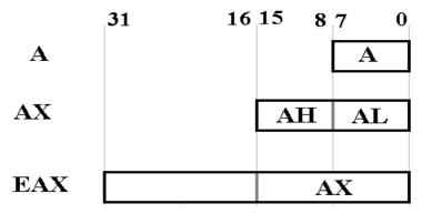
Structure of the EAX register in the Intel 80386. There is no name for the high–order 16 bits of EAX. The AX, AH, and AL registers can all be referenced directly.
