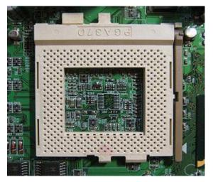
The socket is a ZIF (Zero Insertion Force) type, designed for easy insertion. As noted, it has 370 pin connectors.
