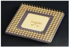
The Intel 80486 had 196 pins arranged as a hollow rectangle. It should be obvious that it required more than a DIP socket.
