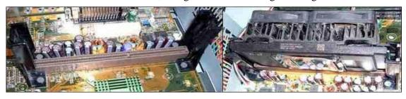
Slot 1 connector is 5.23" long (13.29 cm). Besides the actual connector, the Slot 1 also includes SEC cartridge retention mechanism required to support a processor in SEC cartridge and a heatsink. Maximum supported weight of the processor with the heatsink is 400 grams.
