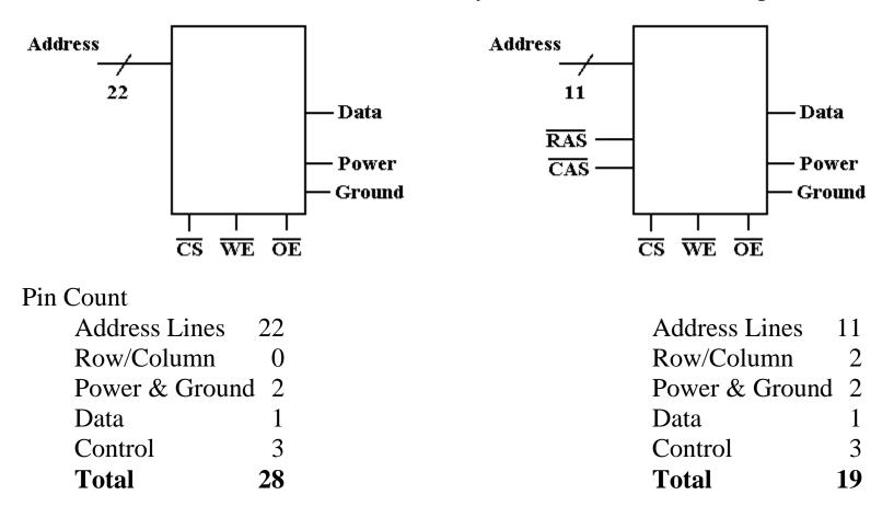
Separate row and column addresses require two cycles to specify the address.
