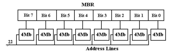
For applications in which data integrity is especially important, one might add a ninth chip to hold the parity bit. This reflects the experience that faults, when they occur, will be localized in one chip.
