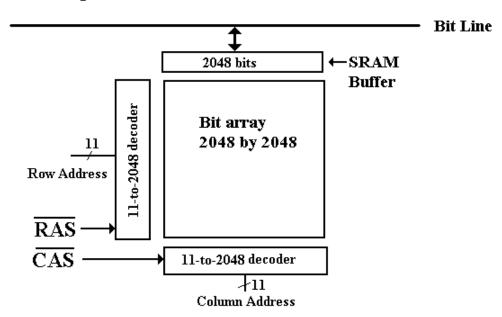
In a modern scenario for reading the chip, a Row Address is passed to the chip, followed by a number of column addresses. When the row address is received, the entire row is copied into the SRAM buffer. Subsequent column reads come from that buffer.
